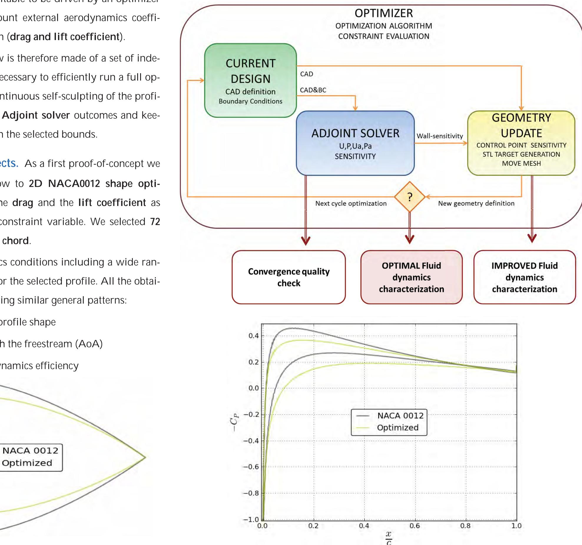
We tested several fluid dynamics conditions including a wide range of Angles of Attack (AoA) for the selected profile. All the obtained results were coherent, showing similar general patterns:
